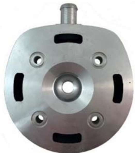
PHOTO OF THE COMBUSTION CHAMBER IN THE CYLINDER HEAD
