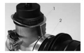
f) Only one rubber gasket is allowed to be used in the carburetor cap.
