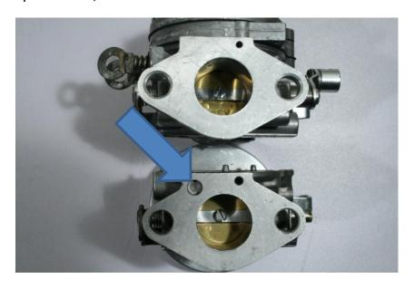
2. An "old " non compliant carb (on the left) has a recess around the dump tube.
