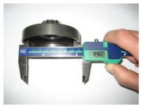
The inner diameter has to be measured with a sliding calliper. The measurement has to be done in the middle of the clutch drum (in the contact area of the clutch drum). Maximum diameter: 84.90 mm.
