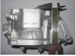
All transfer ports and passages have cast finish surface except some removal (done by the manufacturer) of cast burr at the inlet passage. and exhaust port and passages. All ports have chamfered edges to prevent ring snagging. Any additional machining is not permitted. The top edge of exhaust port may show some preexisting machining from the manufacturer. The sealing flange for the exhaust socket may show signs of machining from the manufacture.
