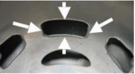
On cylinders marked 223 993 the upper edge of the central boost port may show factory machining.
