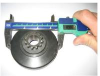
Diameter has to be measured with a sliding caliper just beside the radius from the shoulder (not at the open end of the clutch drum).
