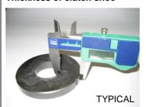
Measurement has to be done at the 3 open ends of the clutch shoes, 5 - 10 mm from the machined groove (all clutch shoes must be completely closed at measurement - no gap).
