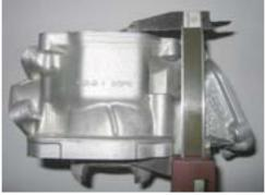
All transfer ports and passages have cast finish surface except some removal (done by the manufacturer) of cast burr at the inlet passage. and exhaust port and passages. All ports have chamfered edges to prevent ring snagging. Any additional machining is not permitted. The top edge of exhaust port may show some preexisting machining from the manufacturer. The sealing flange for the exhaust socket
