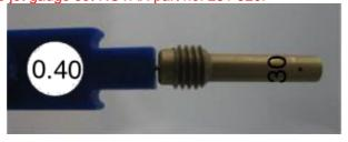
17.15.3 Plug gauge 0.40mm may NOT enter one of the 4 cross bores of the idle jet insert 30. (Use jet gauge set ROTAX part no. 281 920)
