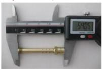
Length of bottom section of needle jet: 11.50 +/- 0.2mm 17.14.2
