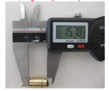
17.18.3 Atomizer, dimension of cutaway: 6.00 +/- 0.15mm
