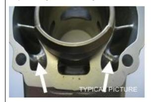
5.7.2 All ports have chamfered edges. Any additional machining is not permitted.
