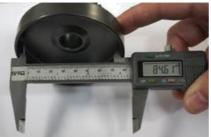
The inner diameter has to be measured with a sliding calliper. The measurement has to be done in the middle of the clutch drum (in the contact area of the clutch drum). Maximum diameter: 84.90 mm.
