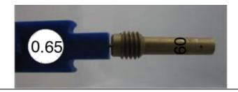
17.16.3 Plug gauge 0.65mm may NOT enter one of the 4 cross bores of the idle jet insert 60. (Use jet gauge set ROTAX part no. 281 920)
