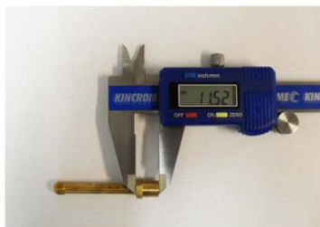
Total Length (Bottom Section): 11.50 +/- 0.20mm
