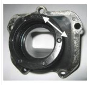
Some factory flash removal may be present at the conjunction of the inside contour and the carburetor stop mounting face. This is a manual trimming operation consisting of a small corner break of less than 3 mm in width. No additional grinding or machining is permitted.
