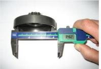
The inner diameter has to be measured with a sliding calliper. The measurement has to be done in the middle of the clutch drum (in the contact area of the clutch drum). Maximum diameter: 84,90 mm.
