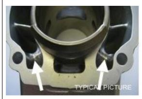
5.7.2 All ports have chamfered edges. Any additional machining is not permitted.
