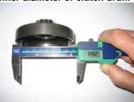
The inner diameter has to be measured with a sliding calliper. The measurement has to be done in the middle of the clutch drum (in the contact area of the clutch drum). Maximum diameter: 84,90 mm.
