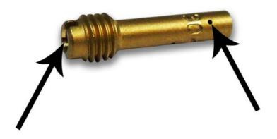
If Pin Gauge 0.015" or 0.40mm fits, then the Jet is ILLEGAL If Pin Gauge 0.015" or 0.40mm fits, then the Jet is ILLEGAL
