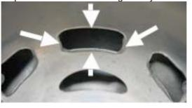
On cylinders marked 223 993 and 223 994 the upper edge of the central boost port may show factory machining.
