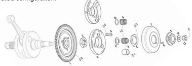
Engines must be fitted with the new needle cage bearing 15x19x17 (item 9) as well as new O-Ring 12 x 2.5 (item 10) only.
