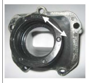
Some factory flash removal may be present at the conjunction of the inside contour and the carburetor stop mounting face. This is a manual trimming operation consisting of a small corner break of less than 3 mm in width. No additional grinding or machining is permitted.
