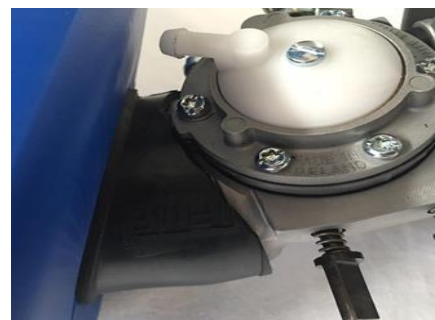
B. Rubber cut in a curved shape to fit around the carburettor top plates
