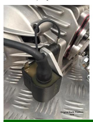
**Photo 2** - Showing the position of the earth hole that Is permitted to be drilled in the crankcase.
