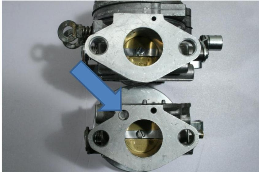
2. An “old “ non compliant carb (on the left) has a recess around the dump tube.
